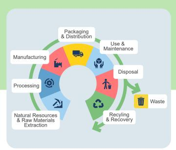
To understand all of the exchanges between the studied system and the environment, you need to map all the processes with their inputs and outputs and how they are interlinked. This map is needed to calculate the overall environmental impact.
